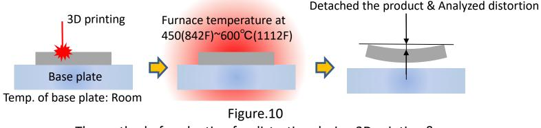
The method of evaluation for distortion during 3D printing & the stipulation of heat treatment for stress relief.
