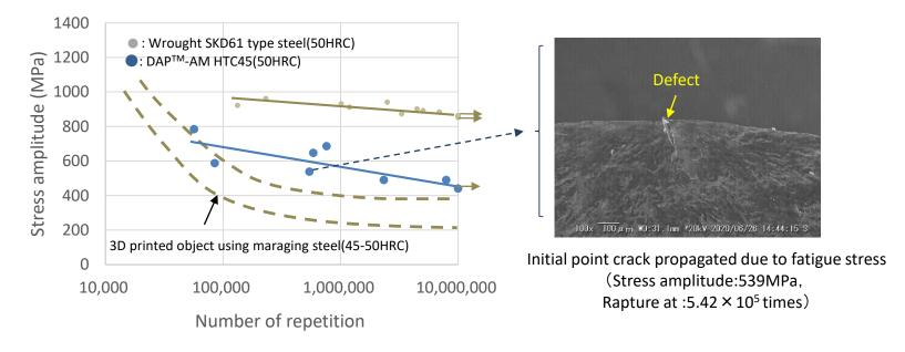
Figure.5 Fatigue strength and typical fatigue fracture surface of DAP<sup>™</sup>-AM HTC.
