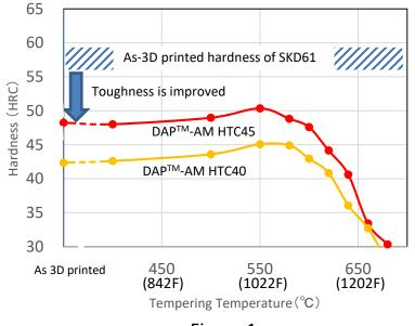
Figure.1 Correlation of the hardness between as 3D printed and tempered after 3D printed. (Tempering(°C) × 1h] twice) The temperature of base plate is 200°C (392F)
