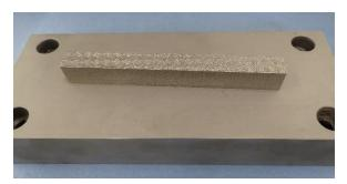
Figure. 11 Appearance of specimen. (DAP<sup>TM</sup>-AM HTC40: 15W × 17H × 150Lmm)
