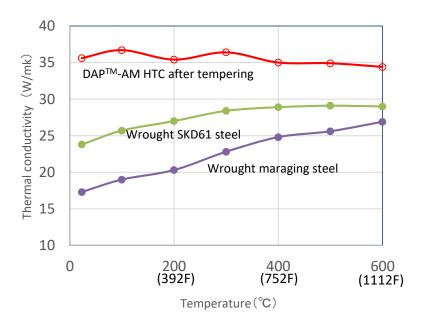
Figure.2 Comparison Table among individual material. (Tested by laser flash method )
